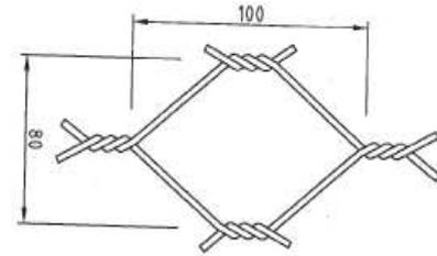
Rockfall protection mesh used as a system to prevent rockfall onto roads and railways. Is used together with rock bolts and other system elements to catch falling rocks from slopes and cuts and prevent falls onto roads and railways.
