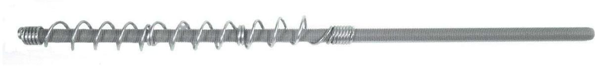
Rock support bolt. The bolt is equipped with a large spiral for safe and controlled mixing of the polyester. The bolt is supplied with a large bevel at one end.
