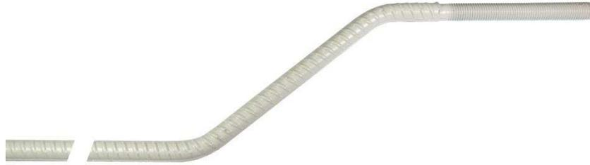
Bolt for suspension of road lighting support ladders. Bolts are normally installed in connecting sleeve M16/M20 B2000-8. The bolt is designed to take up a deviation of up to 150 mm from the centre line. Equipment is clamped to the bolt.
