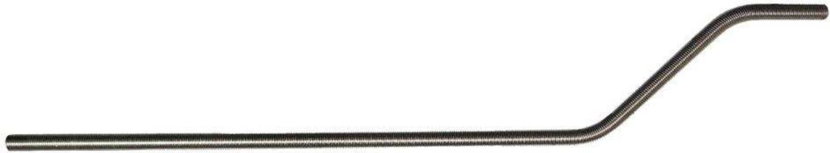
Bolt for suspension of ladders for light fixtures. The bolt is normally mounted in a sleeve / transition sleeve of the same capacity, and is designed to accommodate deviations up to 150mm from the centreline. The equipment is clamped to the bolt or screwed directly to the thread.
