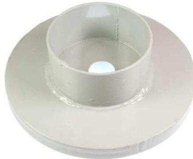
Securing plate for ceiling elements. The plate is mounted on the fixing bolt. The plate has an oval hole, so that the socket can easily be threaded into the recess in the element.
