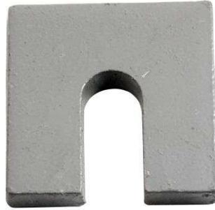
Backing plate used on the rear of concrete wall elements. The plate has a slot which allows the plate to be inserted around the bolt between the nut and wall element.
