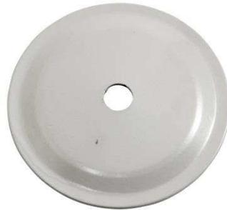
Front washer for PE foam. The washer is entered onto the bolt after the PE foam is installed. The washer is pressed against the PE foam by tightening the nut fitted after the washer. The nut is tightened until the nut is flush with the PE foam. That is, the washer should be pressed slightly into the PE foam. This generates the necessary pressure on the rubber seal on the back plate on the rear of the PE foam and provides a good seal.
