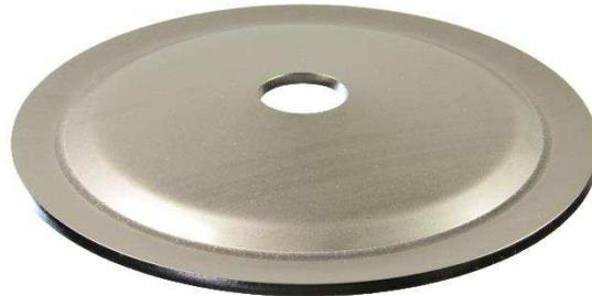
Front washer for PE foam. The washer is entered onto the bolt after the PE foam is installed. The washer is pressed against the PE foam by tightening the nut fitted after the washer. The nut is tightened until the nut is flush with the PE foam. That is, the washer should be pressed slightly into the PE foam. This generates the necessary pressure on the rubber seal on the back plate on the rear of the PE foam and provides a good seal.
