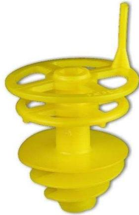
For use in attaching reinforcing mesh to PE foam. The seat ensures 25 mm of concrete cover between the mesh and PE foam. In addition, the seat has an indicator for 80 mm, alternatively 70 mm, to ensure the correct thickness of sprayed concrete. The seat is mounted at mesh intersections.
