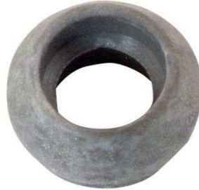
Sealing plug to ensure watertight bolt insertion through back plates. The sealing plug is pre-mounted on the back plate. In order for the sealing plug to function as intended, it is important that the plug is not pulled back and forth on the bolt. If the sealing plug is damaged it can be easily replaced with a new one.
