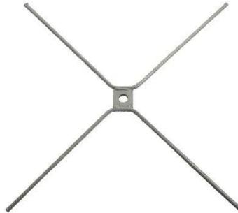
Reinforcement fitting for use with bolts for PE foam. The fixture is mounted on the bolt after assembly of the reinforcement mesh, helping to keep the mesh in place during sprayed concrete application.
