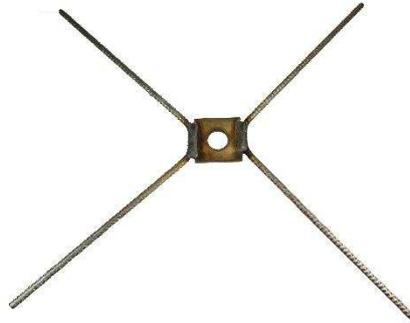
Reinforcement fitting for use with bolts for PE foam. The fitting is mounted on the bolt after assembly of the reinforcing mesh, helping to keep the mesh in place during sprayed concrete application.
