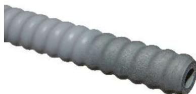
Fully threaded self-drilling anchor bar. For slope stabilization, various mountain rock anchorages also for tunneling. The anchor bars are usually used in demanding geological conditions with mounted drill/clay bit where the anchor bar is drilled in with a simple and flexible joint to achieve the desired length. Can be grouted during drilling or post-grouting.
