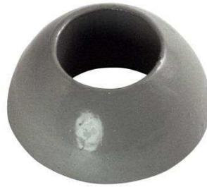
Half ball for use with spherical/triangle bearing plate to achieve a good transfer of forces with angular deviation of the bearing plate in relation to the bolt. This prevent bending stress on the bolt.
