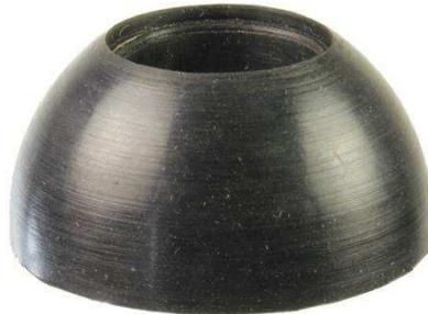
Half ball for use with  $\varnothing 150$  or  $\varnothing 190$  spherical bearing plate to achieve a good transfer of forces with angular deviation of the bearing plate in relation to the bolt. This prevent bending stress on the bolt. The rubber coating aids waterproofing from both sides of the PE foam.
