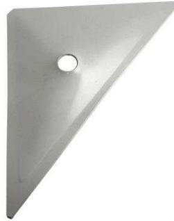
Bearing plate for use with Ø50 half ball for installation of M20 and M24 rock support bolts in cracked rock. The bearing plate is capable of taking up angle deviations of up to 25°.
