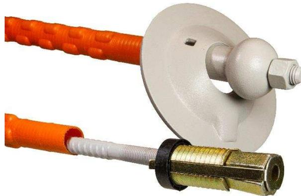
NC-Bolt M22 combination bolt for rock anchoring. The bolt is used with an expansion shell for immediate work safety support. The bolt is subsequently grouted for permanent anchoring.
