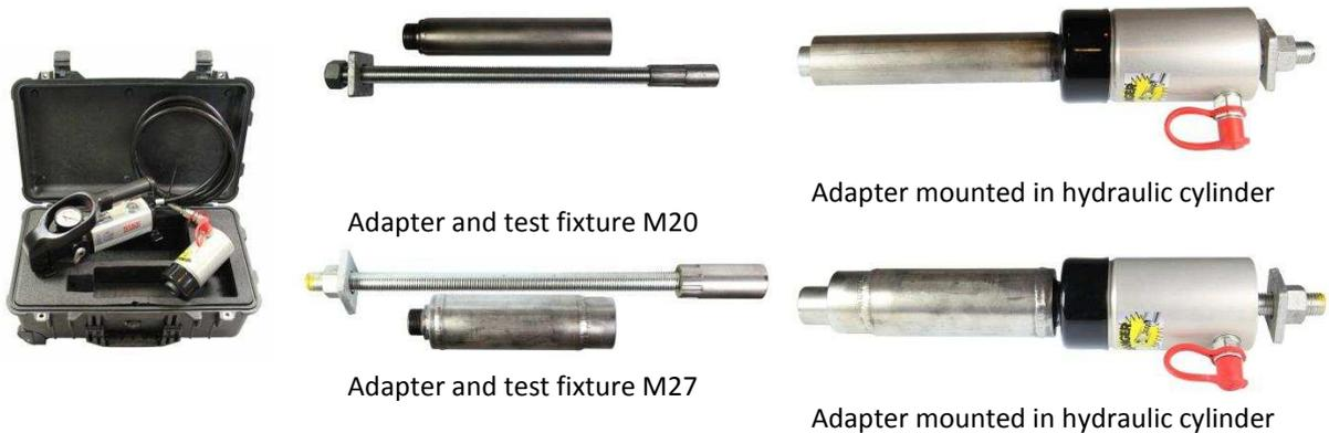
Tool kit for tensile testing of M20 Rebar Bolt and M27 Combination Bolt when anchored or grouted into boreholes. The tool is small, lightweight and easy to use. Supplied in an impact-resistant plastic toolbox. The kit is easy to carry onto the work platform when testing bolts. Bolts are pull tested to specified requirements. Normal requirement for work safety rock support bolts is 50 kN (5 tons). See also handbook R761 Statens Vegvesen.
